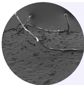
Zinc whisker: Scanning electron microscope (SEM) image of zinc whiskers on the surface of EZ-coated steel wire
